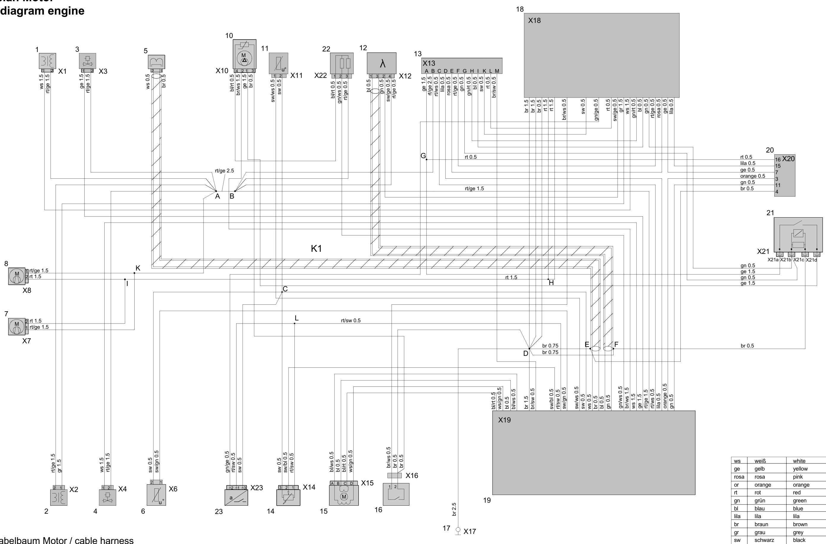
**Schaltplan Motor / Wiring diagram engine**
